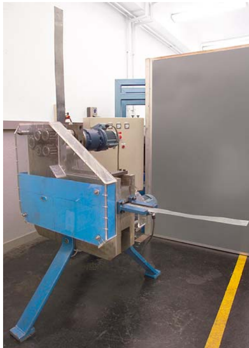
Fig. 1 Machine for ECAP of aluminum sheet at Monash University
